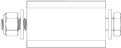
1/4" X 2-1/2" Hex Bolt - 1/4" Flat Washer (x2) - Spacer Square - 1/4" Nylock Nut
