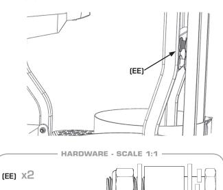
1/4" X 1-1/2" Hex Bolt - 1/4" Lock Washer - 1/4" Flat Washer (x2) - 1/4" Spacer - 1/4" Nyloc Nut
