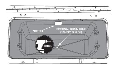
Make sure the Bin rests inside the Bin Ridge in the Seat Base. Install the self-tapping Screws thru all holes in Bin into the Seat Base.
