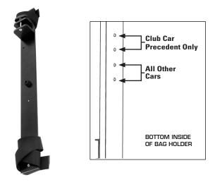
Thread **(EE)** thru Safety Bar cross brace slot, then into the lowest hole set for your Car Model.
