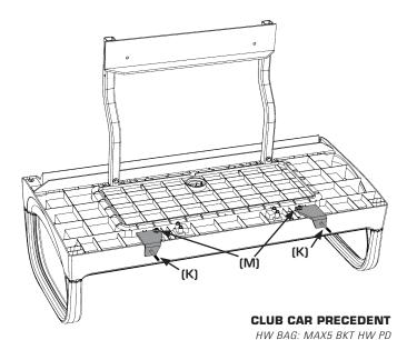
\*\*Insert bolts (K) before attaching brackets\*\*
