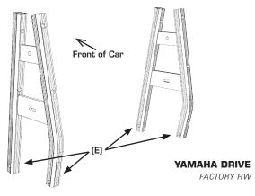
(E) x4 REUSE FACTORY HARDWARE FROM BAG RACK REMOVAL
