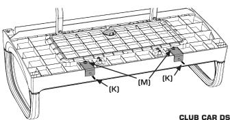
\*\*Insert bolts (K) before attaching brackets\*\*
