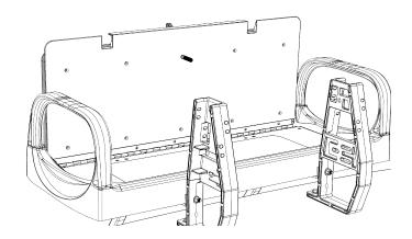
Loosely screw in all four corner holes first, then screw in the remaining vacant holes.
