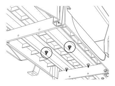
Place Hitch Receiver (**JJ**) over Bolts and reinstall the Washers and Nuts. **NOTE:** Fully tighten Hardware.
