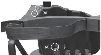
Attach the Universal Seat Back Plates to the Seat Back Supports using 1/4" x 1-3/4" FHP Bolt, 1/4" Flat Washer (back), and 1/4" Nyloc Nut (2x both sides — through top and bottom holes marked RXV).
