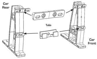
Attach the Seat Back Plates to the rear Seat Back Supports using 1/4" x 1-1/4" FHP Bolt, 1/4" Flat Washer (back), and 1/4" Nyloc Nut (2x both sides through holes marked CC-P).
