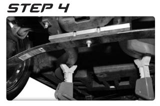
Place lift block between leaf spring and frame.
