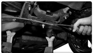
Pry the leaf spring away from the cart to allow enough clearance for the lift bar.
