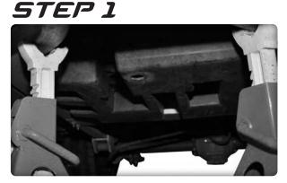
Place RUN/TOW switch in TOW position. Chock wheels and lift cart. Place cart on jack stands as shown.
