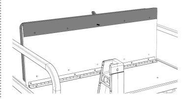
Loosely screw in all four corner holes first, then screw in the remaining vacant holes.
