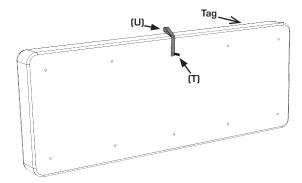
BOTTOM CUSHION HW RSK CUSH PAT Angle Seat Bottom Plastic upright to 90° and insert 2/1 Seat Bottom Cushion and the flip angle in the top center hole using the Temporary Stud.
