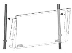
Snap Extrusions & Windshield onto front frame, then slide until Windshield sits on grommet.
