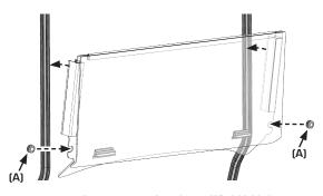
Insert grommets into slots on Windshield, then snap Extrusions & Windshield onto front frame.
