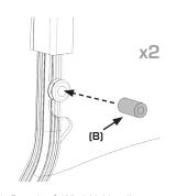
Slide Extrusion & Windshield until grommet aligns with hole in frame, then insert spacer.
