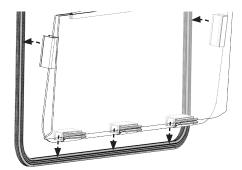
Push in and down at the same time to snap the Extrusions & Windshield onto the front frame.
