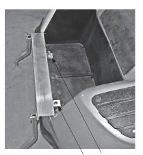
1) Mount Bumper Channel over bumper. Align Bumper Channel tabs with original holes in the car bag well and install.
