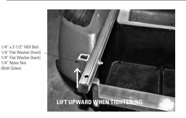
1) Connect the cargo bed upright supports to the seat back/base supports. The upright supports should be on the outside of the base support. NOTE: when tightening bolt, lift upward on the base support to make it flush with the top of the upright support.
