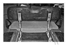
1) Install the factory seat back cushion. Once the seat back is installed, fully tighten seat back bolts only.
