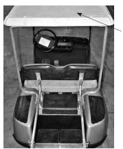
2) Align factory top with front frame and rear struts. Reinstall top using the original top hardware. Do not fully tighten hardware until all bolts have been installed.
