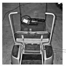
1) Mount rear strut kit to seat back/base supports. NOTE: Rear strut kit is NOT
