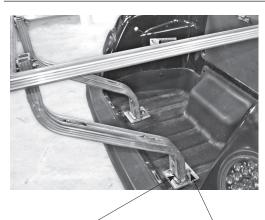
Mount each cargo bed support to the car, using the holes that were drilled in the bagwell floor from **STEP 1C**.
