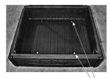
Align the four holes in cargo bed with the four holes in the cargo bed frame. Mount cargo bed using stainless steel hardware on top. 5/16" x 3-1/4" SS HEX Bolt 1" SS Washer (top) 5/16" Flat Washer (bottom) 5/16" Nyloc Nut (bottom) (2x Both Sides)
