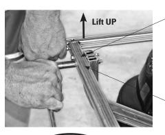
When tightening, lift UP on cargo bed frame to make it flush with the top of the cargo bed support legs.
