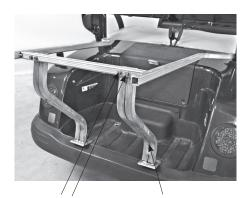
1/4" x 2-1/2" Hex Bolt<br/>1/4" Flat Washer (front)Attach the cargo bed support1/4" Flat Washer (rear)legs to the back of the cargo bed1/4" Nyloc Nut<br/>(Both Sides)frame cross bar. Hand-tighten<br/>hardware only.
