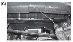
Under the bag well, Locate the steel bar running from side-to-side. Find the two existing holes in the bar. Using these holes as a guide, drill a 5/16" hole up thru the plastic floor in the bag well **(Fig. 1 C)**.
