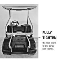
3) Fully tighten rear struts to the cargo bed frames.
