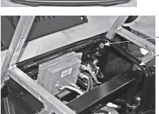
1) Place cargo bed frames into holes where the bag rack was removed.
