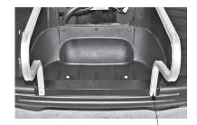
Attach the cargo bed frames to the the Bumper Angle. Attach to the second hole from each outside edge of the Bumper Angle. Hand-tighten hardware only.
