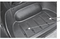
**1)** Remove the plastic button caps in bottom of the bagwell. This will expose an existing threaded hole set.
