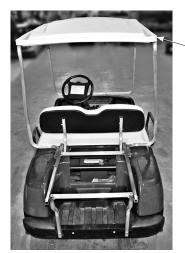
NOTE: The rear strut will have two holes drilled thru tubing. Use the SECOND HOLE from end
