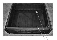
1) Align the four holes in cargo bed with the four holes in the H-frame. Mount cargo bed using stainless steel hardware on top.
