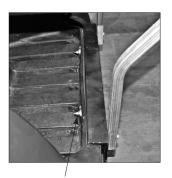
1/4" x 3-1/2" PHP Bolt (Pan Head Phillips) 1/4" Flat Washer (angle side) 2" Plate Washer (inside bumper) 1/4" Flat Washer (bumper side) 1/4" Nyloc Nut (Both Sides)
