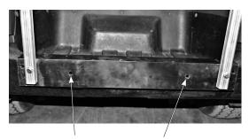
1) Center Bumper Angle on car bumper. Using one of the two holes in the center of the Bumper Angle as a guide, use a 5/16" drill bit and drill completely thru the bumper. Install mounting hardware. Repeat for other remaining hole.
