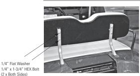
Align the holes in factory seat back cushion with the holes in aluminum seat back supports and install with appropriate hardware.
