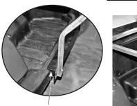
1) Rest the Bumper Angle/Cargo Bed Upright Support Assembly on top of the bumper.
