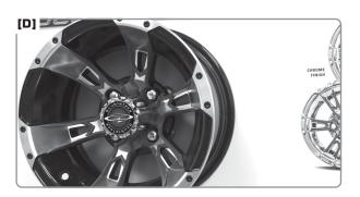
**D]** Align the Wicked Wheel Insert and snap into Wheel. Snap Hub Cap into the Wicked Wheel Insert and install decal.
