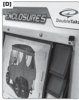
D] Slide Enclosure Cover Flap into the front track of Enclosure Rail.
