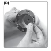
D] Position the Hub Adapter over exposed screw and extra support that was installed above. Next, install the large Fender Washer.
