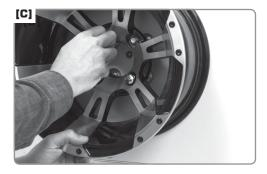
**C]** Position the Wheel onto the protruding bolts. Secure the Wheel with 4 Lug Nuts.
